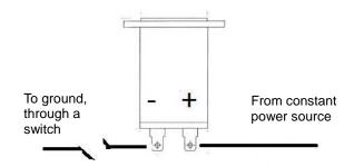
Switched ground can be in the form of a normally open pressure switch (that close when engine is running) or other ground source that is active only when engine is running. Read these instructions thoroughly before installation. Do not deviate from assembly or wiring diagram. Always disconnect battery round before making any electrical connections.
