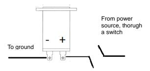
Switched power can be sourced from Igntion Switch, ignition system or other 'hot' source when engine is in operation.
